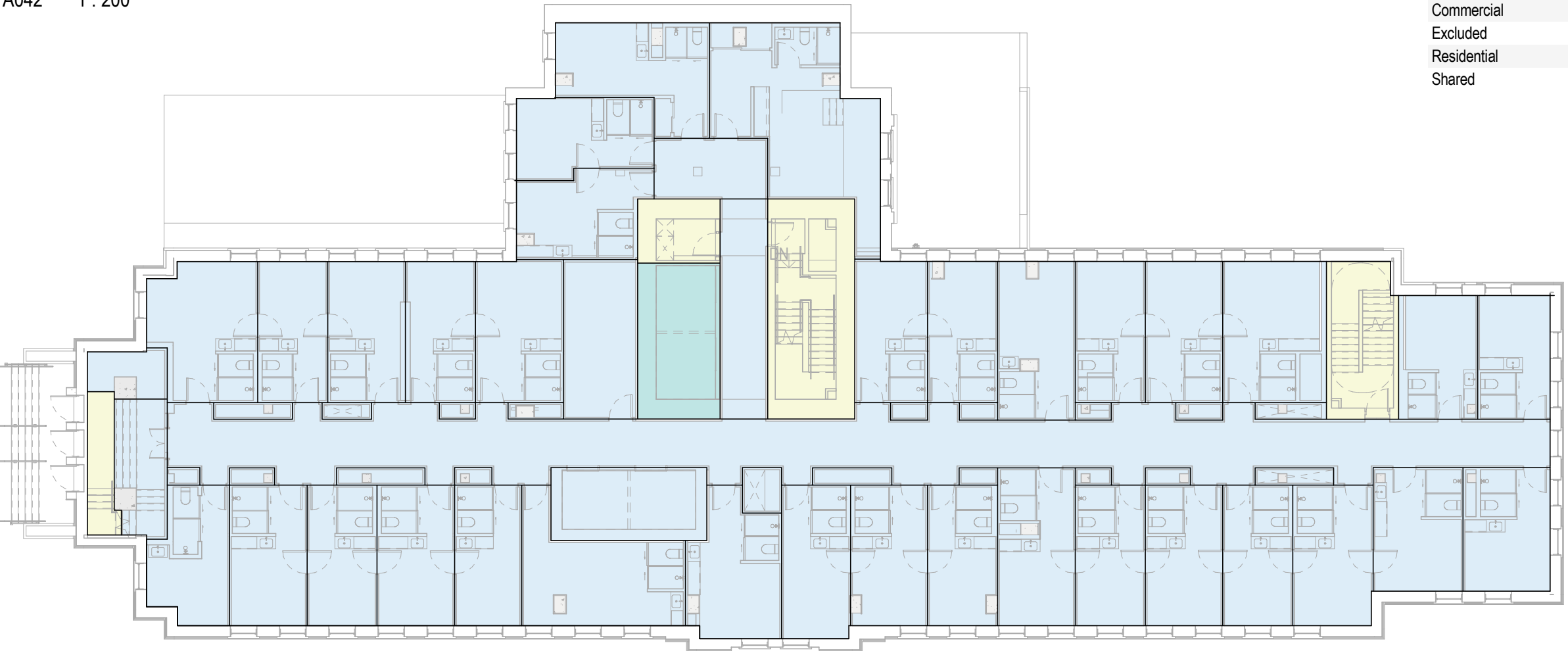
2 Level 02 Floor Area Overlay A042 1:200
