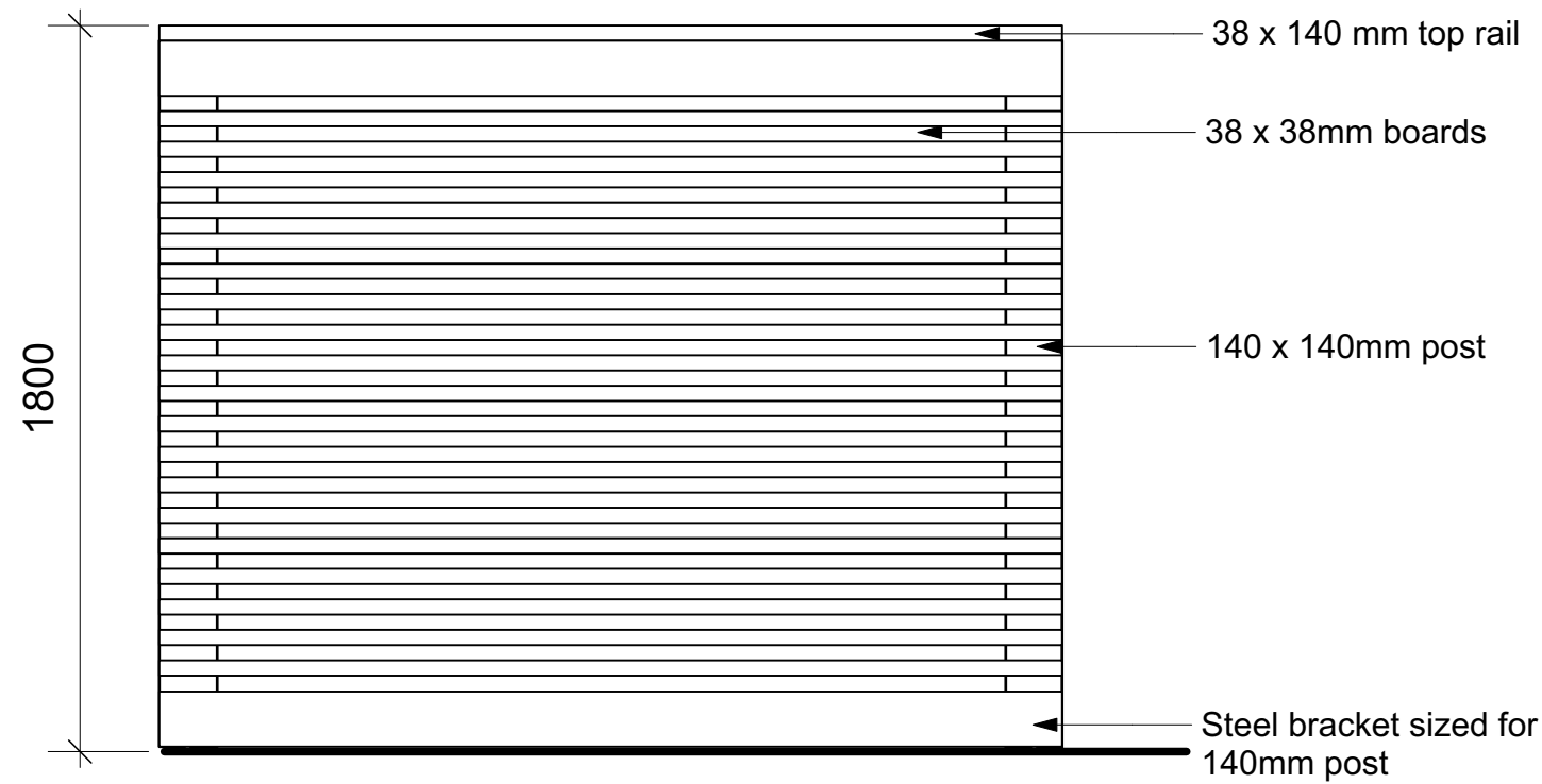
6 1.8m ht. Timber Perimeter Fence Scale: 1:20
