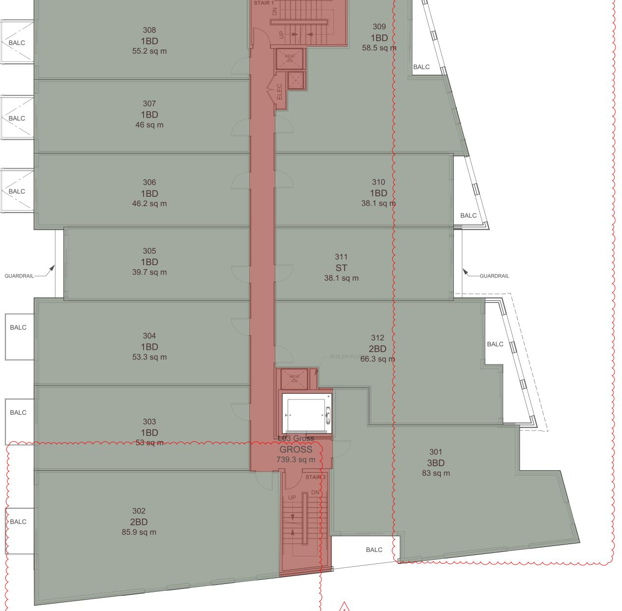
LEVEL 02 - FSR AREA PLAN / SCALE: 1:100
