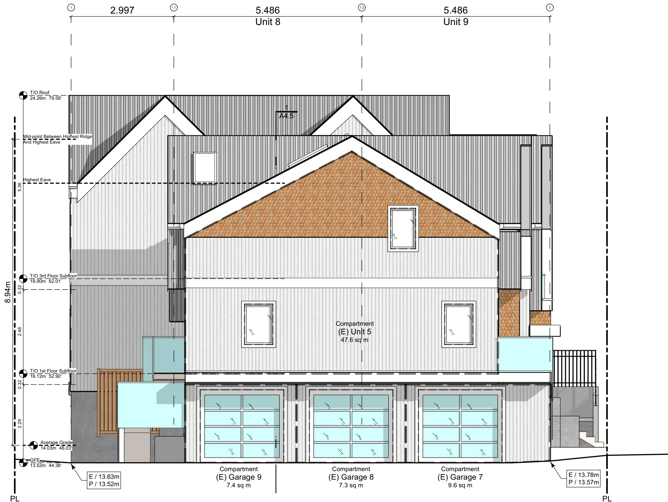
2 East Elevation - Driveway
