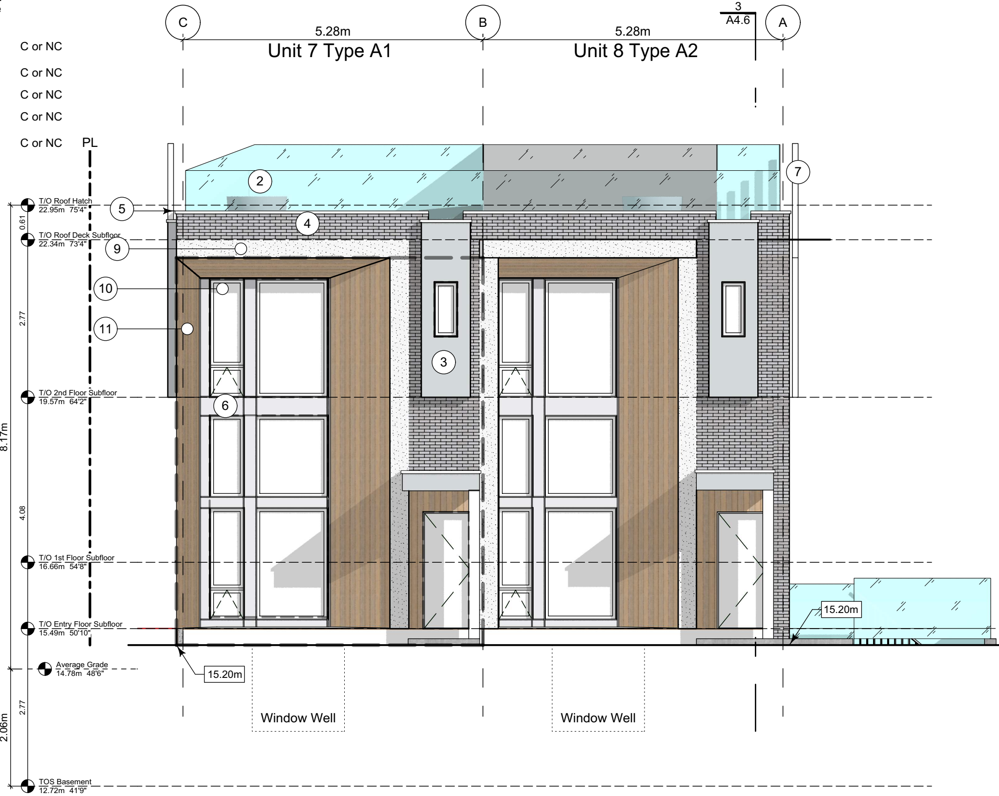
4 West Elevation - Fairfield Road Scale: 1:65
