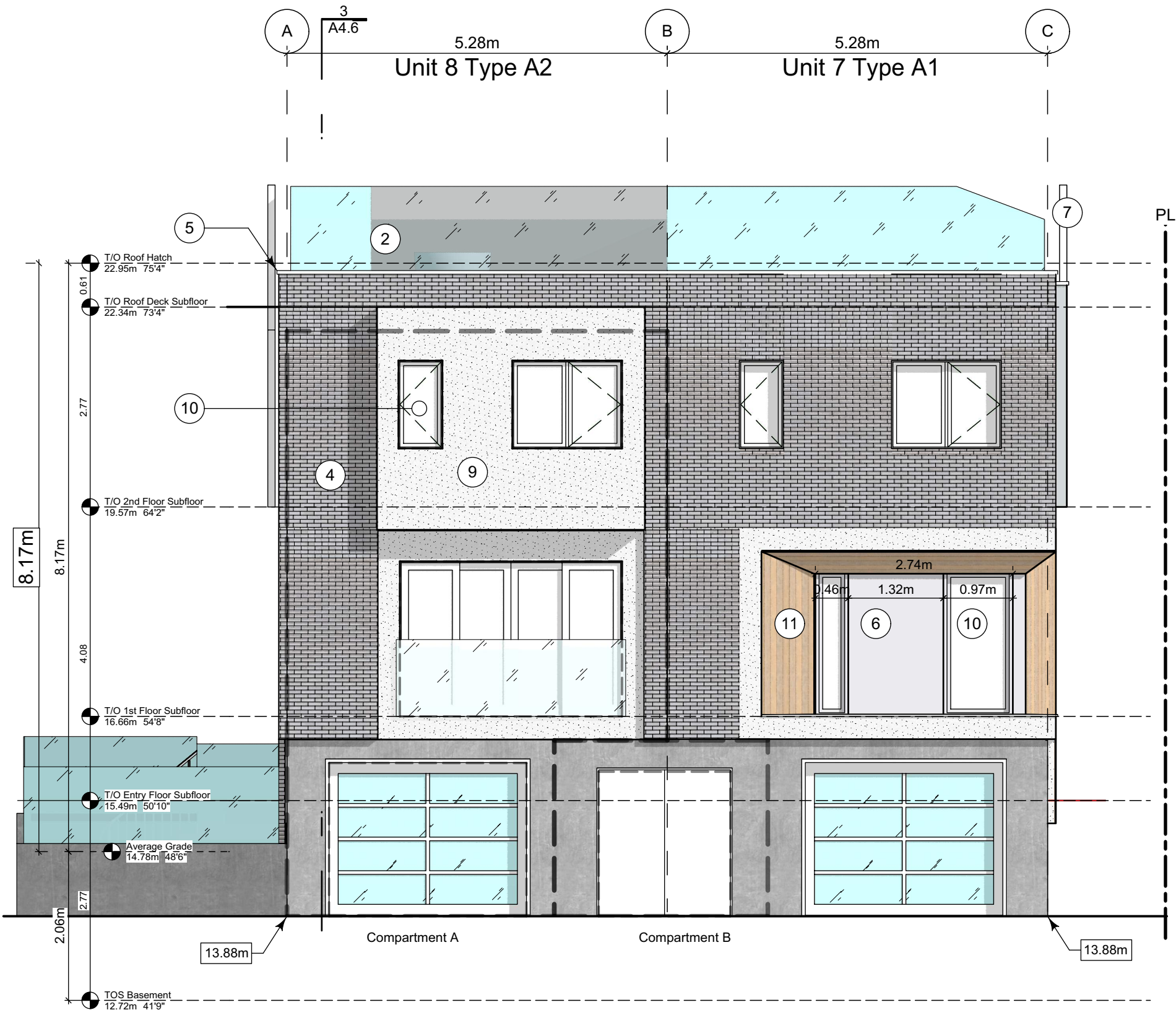
3 East Elevation - Driveway Scale: 1:65
