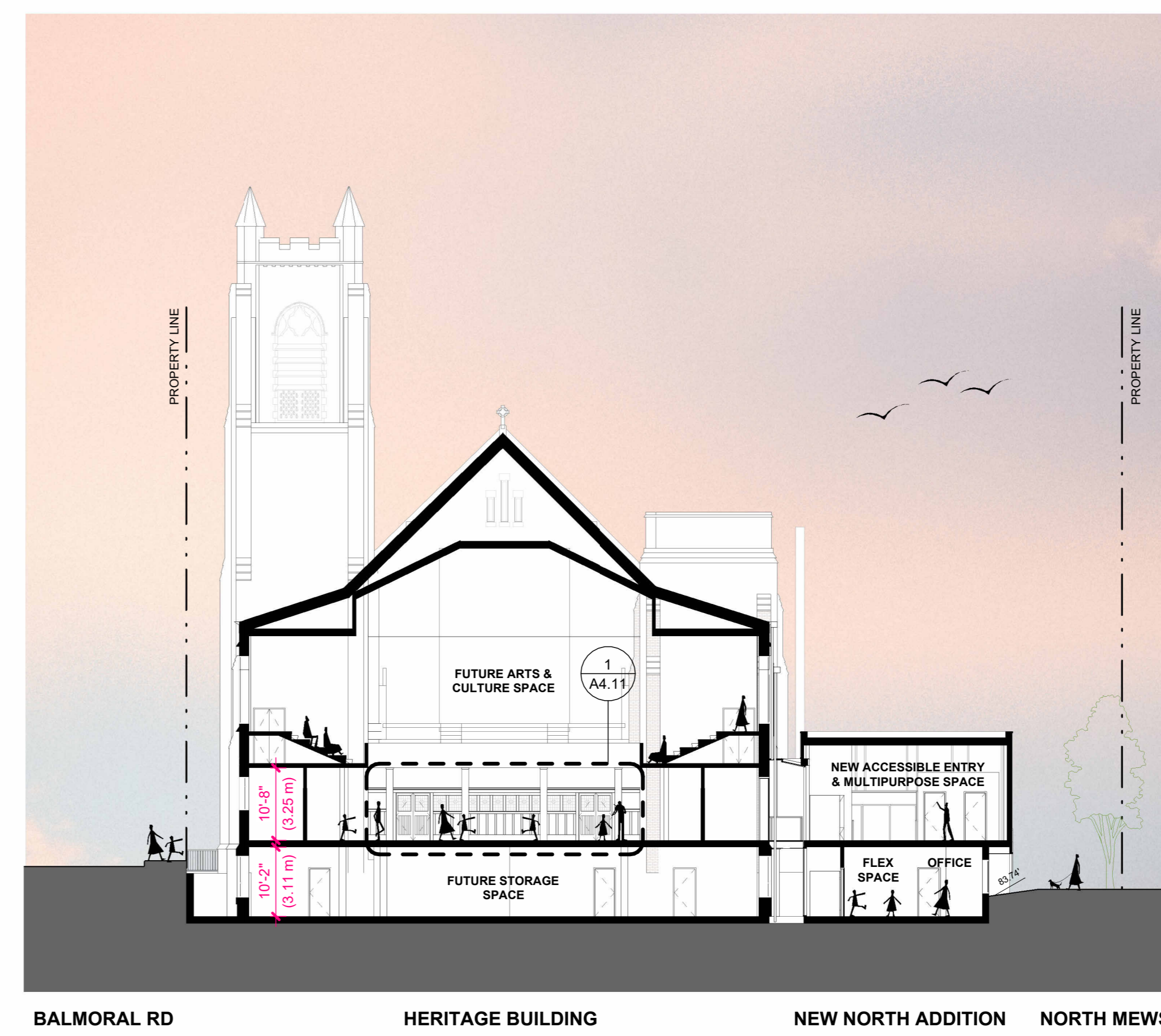
4 SITE SECTION THROUGH HERITAGE BUILDING LOOKING WEST
