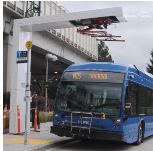
Example of transit vehicle overhead electric charging system at New Westminster's 22 nd Street Skytrain Station (Image source: TransLink).
