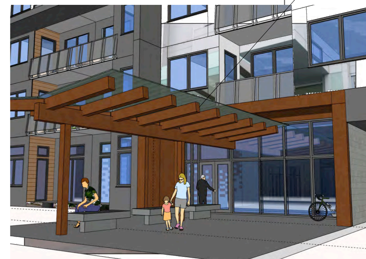
Heavy Timber and Glass Entrance Canopy
