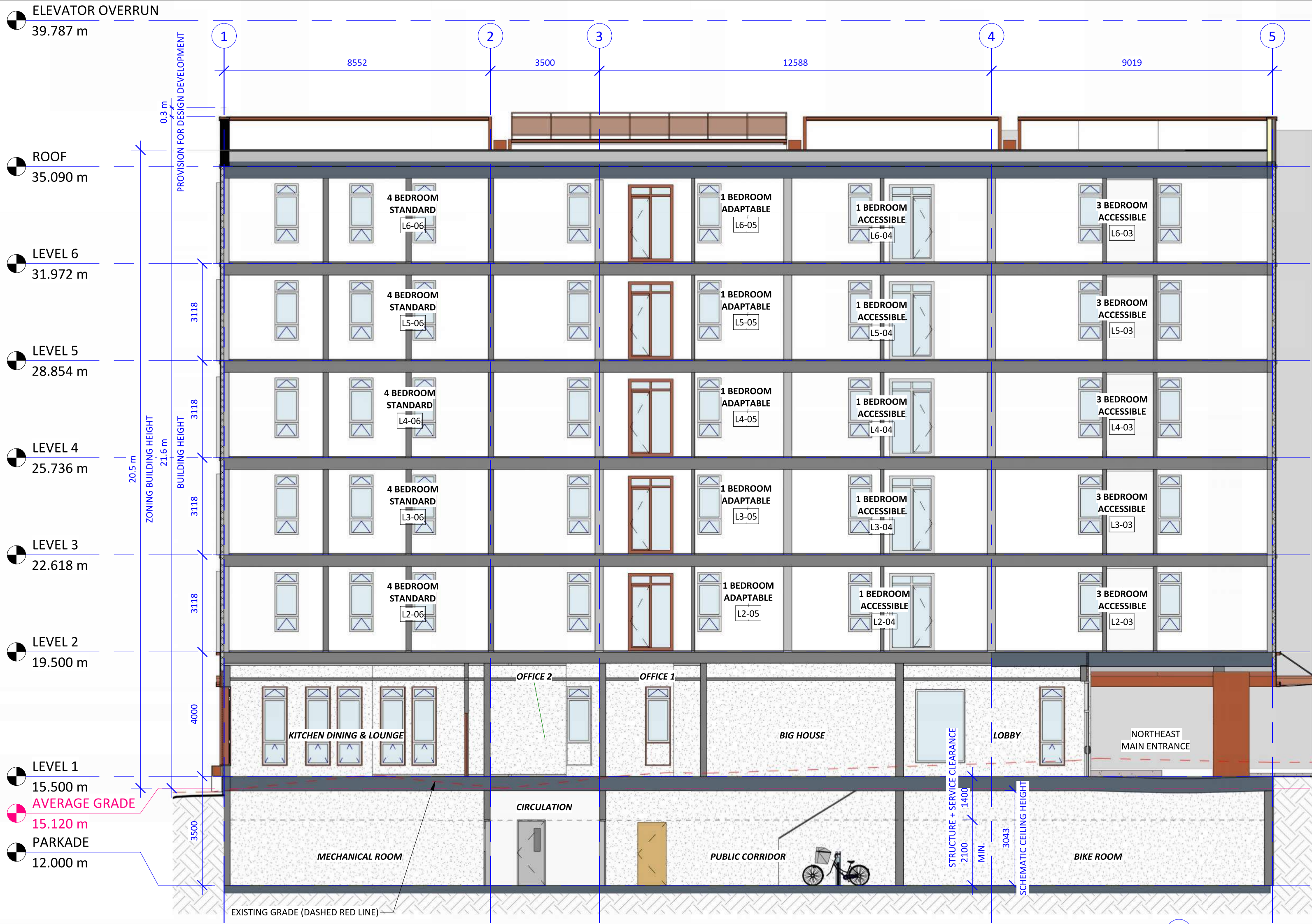
1 EAST - WEST SECTION THROUGH BUILDING 1 : 100
