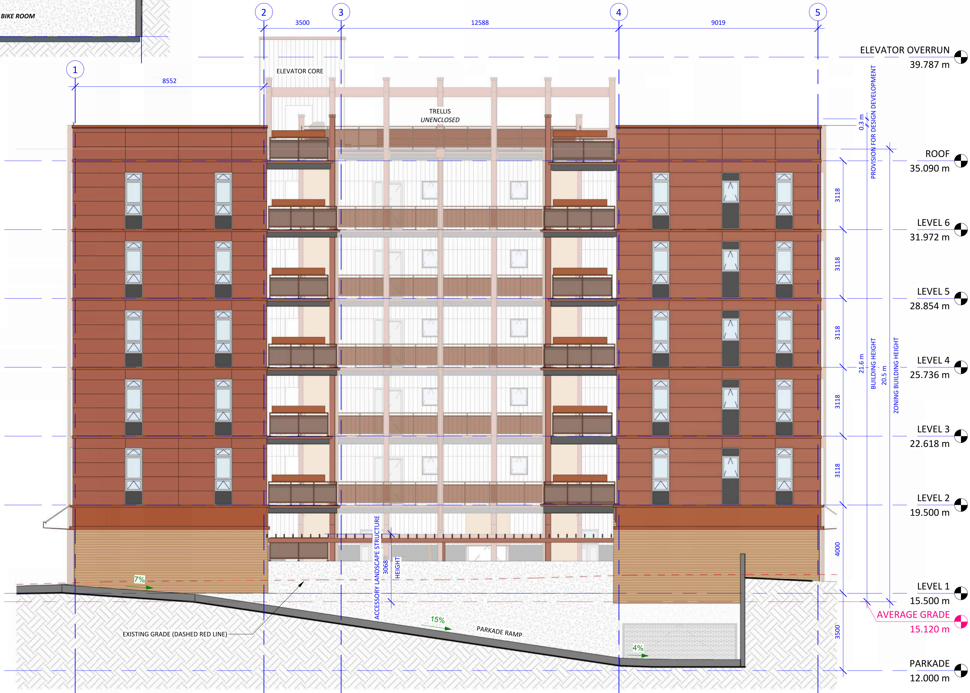
2 EAST - WEST SECTION THROUGH PARKADE RAMP 1 : 100
