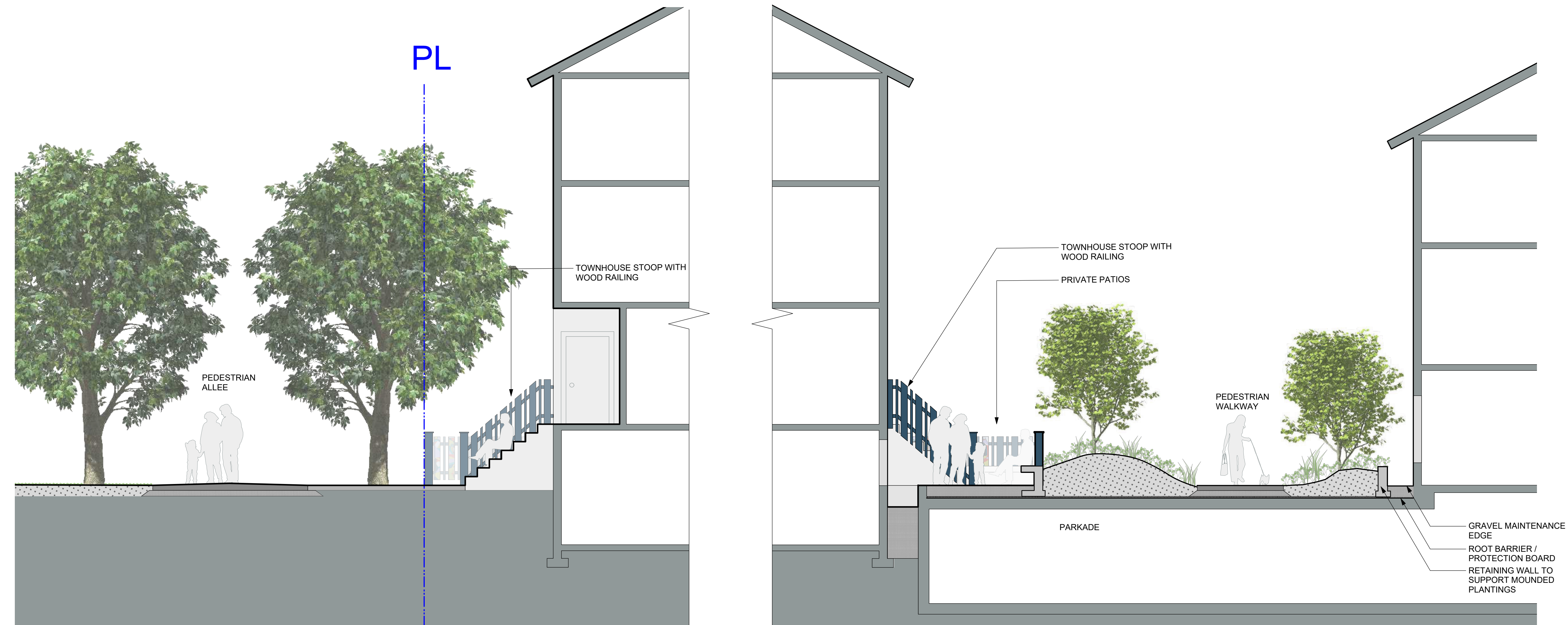
1 Section at Pedestrian Allee and Townhouses Scale: 1:50
