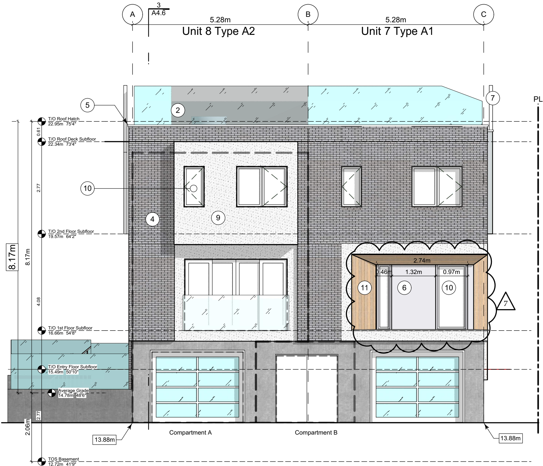
3 East Elevation - Driveway Scale: 1:65
