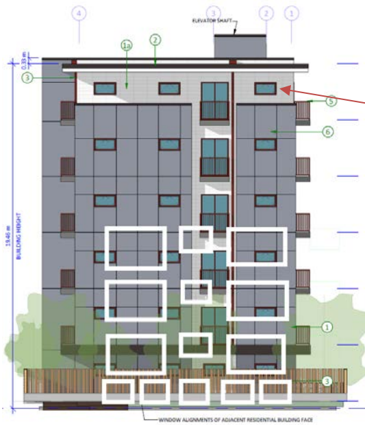
Figure 1: North Elevation of 1042 Richardson St. with window overlay of 1035 McClure St. (white)
