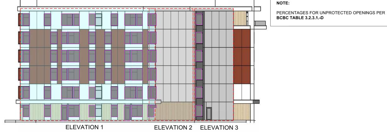
CODE ELEVATION - SOUTH VIEW A012 Scale: 1:200
