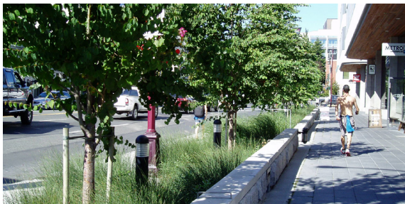
Rain gardens manage and clean rainwater while creating buffers between pedestrians and moving vehicles
