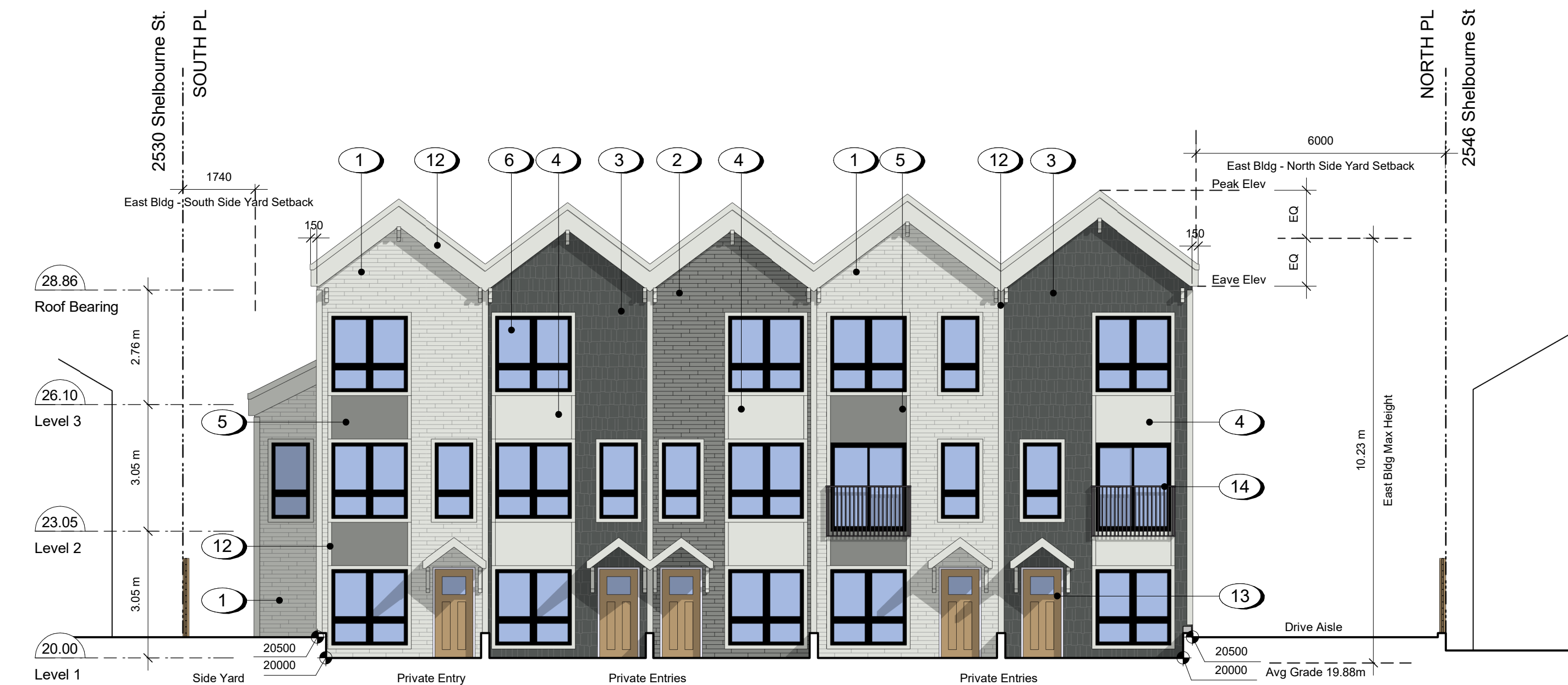
1 East Building - East Elevation A301 SCALE: 1 : 100
