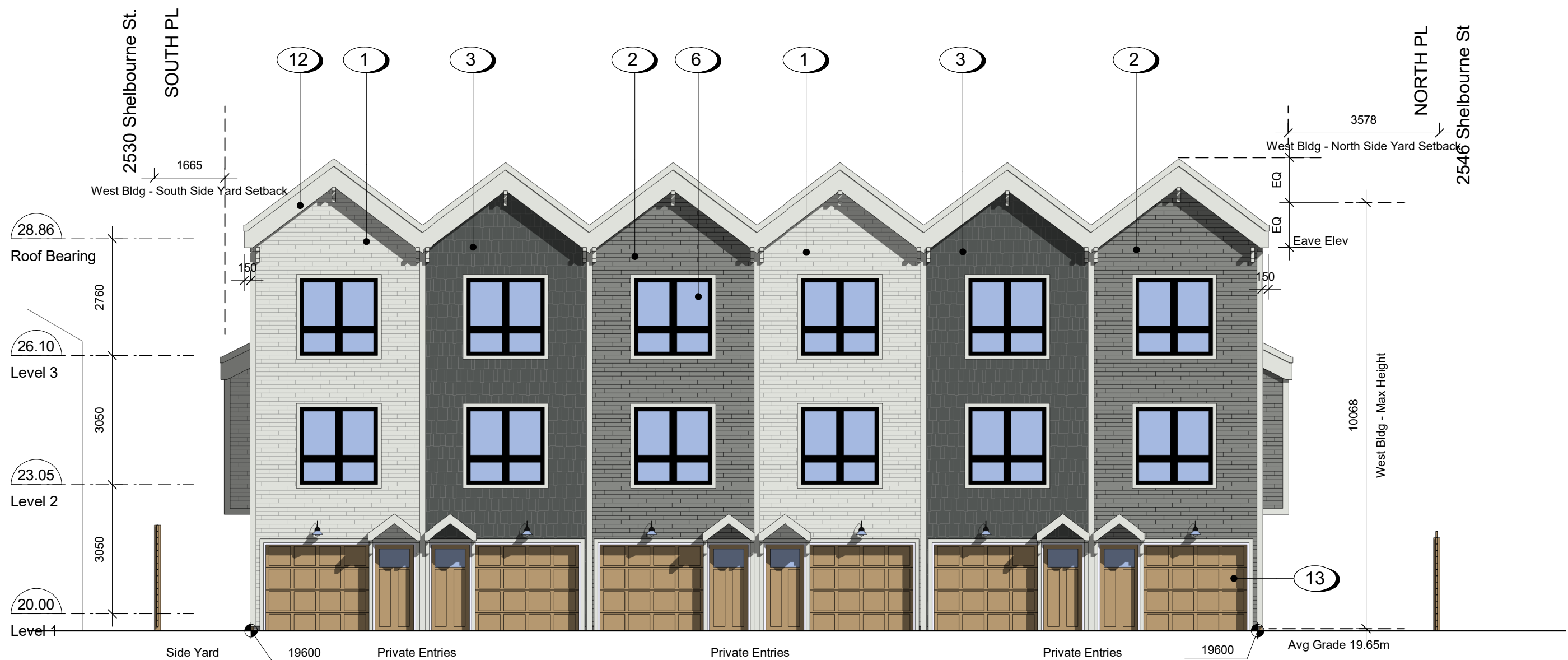
3 West Building - East Elevation A302 SCALE: 1 : 100
