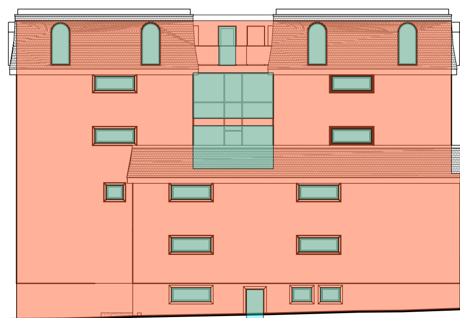
7 South Elevation Scale: 1:200 Table 3.2.3.1-D, BCBC DISTANCE TO PROPERTY LINE = 2.19 m AREA = 378.67 m 2 PROPOSED UNPROTECTED AREA = 49.77 m 2 UNPROTECTED OPENING ALLOWED 16%, 60.27 m 2 PROPOSED OPENING 13.21%
