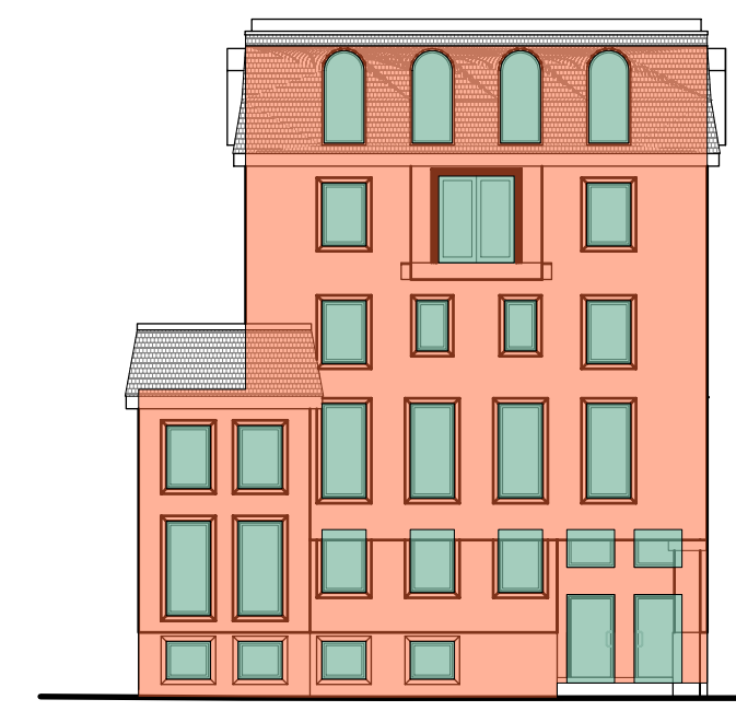
10 Front /East Elevation Scale: 1:200 Table 3.2.3.1-D, BCBC LIMITING DISTANCE = 10.08m AREA = 194.16 m 2 PROPOSED UNPROTECTED AREA = 54.17 m 2 UNPROTECTED OPENING ALLOWED 100%, 194.16 m 2 PROPOSED OPENING 27.90%
