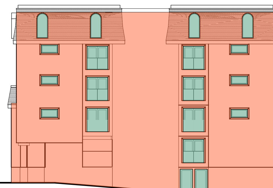
9 North Elevation Scale: 1:200 Table 3.2.3.1-D, BCBC DISTANCE TO PROPERTY LINE = 1.36 m AREA = 381.82 m 2 PROPOSED UNPROTECTED AREA = 48.8 m 2 UNPROTECTED OPENING ALLOWED 14%, 53.43 m 2 PROPOSED OPENING 12.79%
