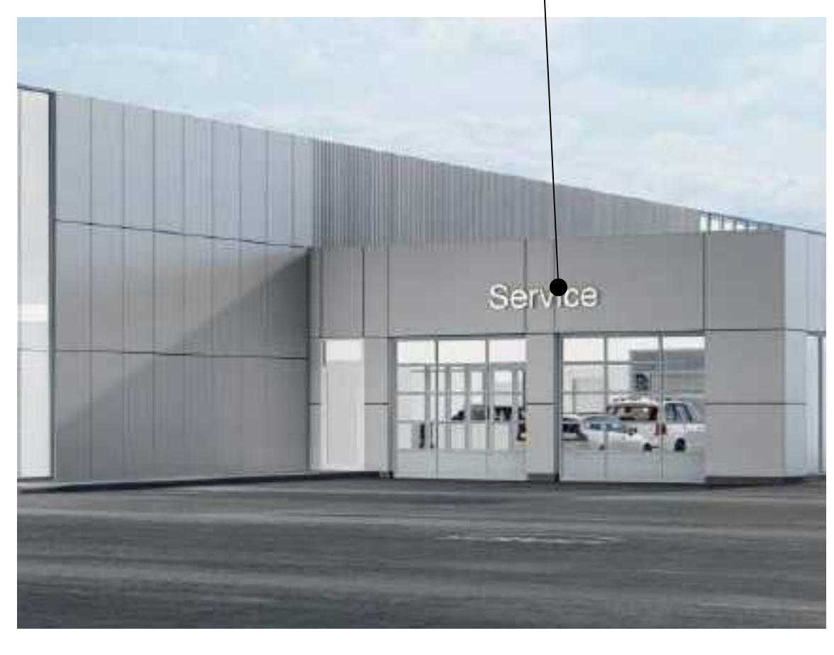
9 Service Letters: Illuminated Channel Letters. Clear Satin brushed aluminum returns. White Acrylic faces with Brushed Silver trimcap. Internally illuminated.
