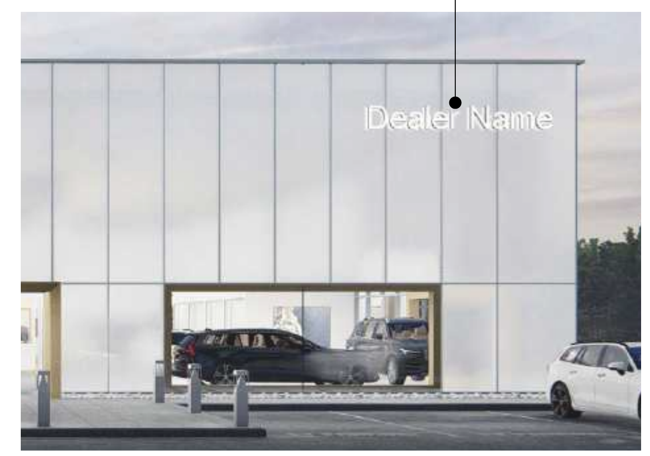
9 Dealer Name: Illuminated Channel Letters. Clear Satin brushed aluminum returns. White Acrylic faces with Brushed Silver trimcap. Internally illuminated.
