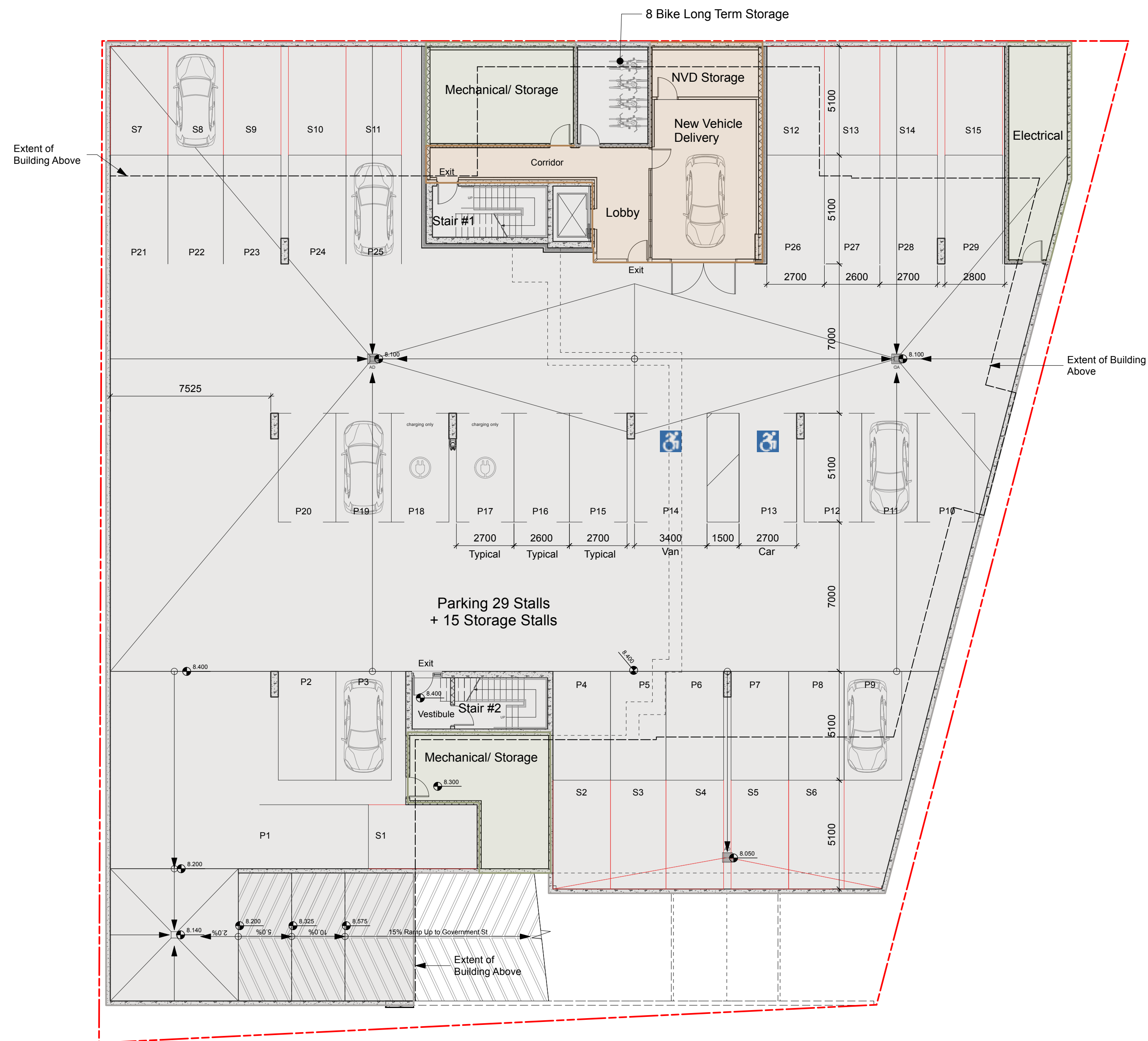
1 P1 Underground Parking Scale: 1:150
