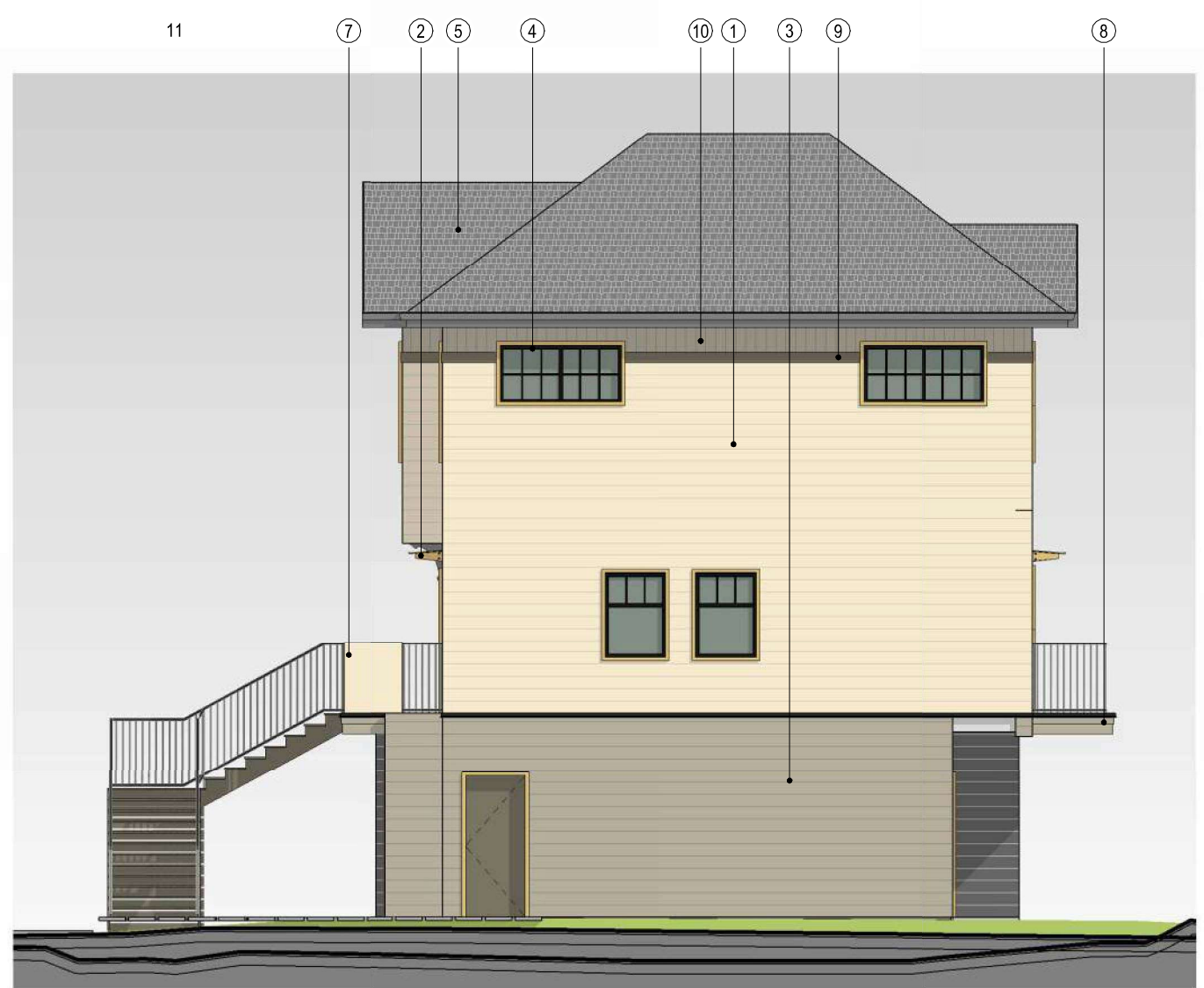
5 WEST ELEVATION - BLDG B 1 : 100
